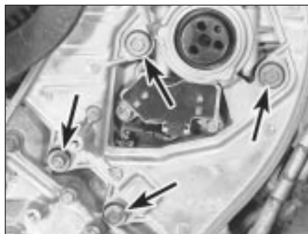
14.2 Front cylinder head backplate retaining bolts (arrowed)
