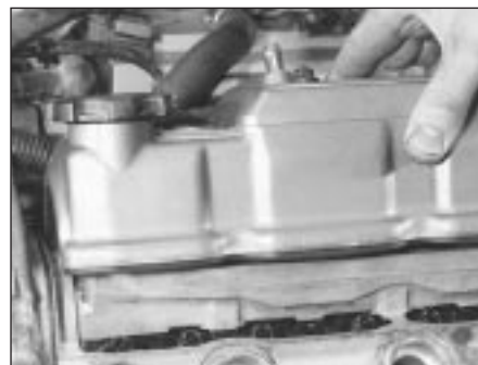
5.5 Lifting off the front camshaft cover
